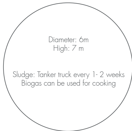
Parameters for the UASB-Reactor
