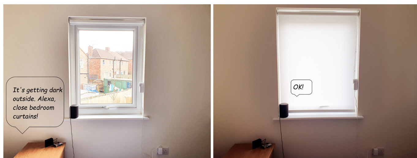
Figure 2: Based on the light level detected by the light sensors, IntraVox will send a command to Alexa to close the bedroom curtains when a decrease in the light intensity is detected. (Ana-Maria Salai)
