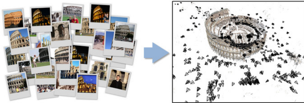
FIGURE 4.6: Structure-from-motion (SfM) - Reproduced from Snavely et al., 2006: It produces 3D scene geometry and camera motion from an unordered 2D image dataset.
