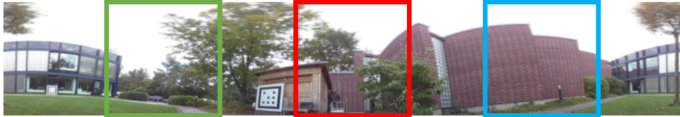
FIGURE 7.13: Generic Landmark-based Localization: The aim of anywhere localization is to use any image patch to estimate the robot's position (x,y) instead of pre-fixed landmarks in a scene. Just like landmarks, these individual patches (i.e., generic landmarks) will give an independent estimate of the robot's position (x,y) .
